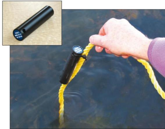
**Figure 3.6. Vemco Minilog-II-T *Submersible Temperature Data Logger* (photo Vemco).**
